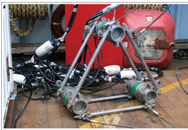
Figure 3. The crew utilized a small air gun as the energy source to illuminate the shallow target hazards. The source was containerized, compressors included, and mobilized on the vessel of opportunity.
