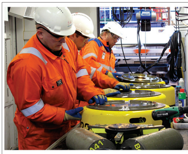
Figure 2. Nodes serviced between retrieval and deployment. The nodes were containerized, deck handling included, and mobilized on a vessel of opportunity. There were two ROVs already on board; one was adapted to handle nodes. Apache chose to use Trilobit nodes for their ability to be containerized and mobilized on the ROV vessel already working in the field.
